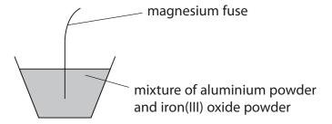
When the magnesium fuse is lit, a very exothermic reaction occurs.
