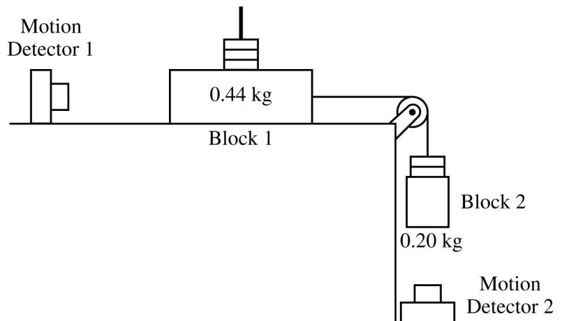
1. Students design an experiment using blocks of adjustable mass to investigate friction using the setup shown. Block 1 of initial mass 0.44 kg is placed on a rough horizontal surface and connected by a string to block 2 of initial mass 0.20 kg. The string extends over a pulley that has negligible mass and friction.
