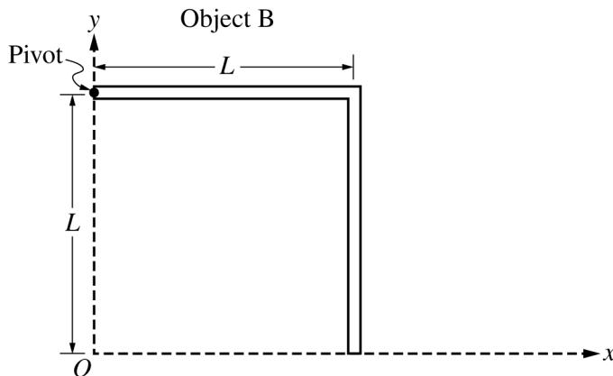
Object B of total mass  $M$  is formed by attaching two thin, uniform, identical rods of length  $L$  at a right angle to each other. Object B is held in place, as shown above. Express your answers in part (b) in terms of  $L$ .
