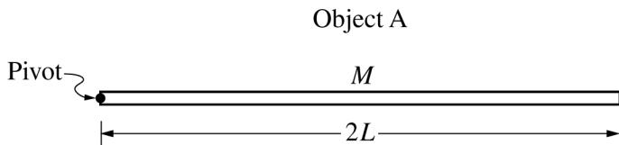
2. Object A is a long, thin, uniform rod of mass  $M$  and length  $2L$  that is free to rotate about a pivot of negligible friction at its left end, as shown above.
